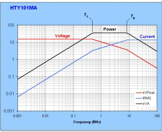
Typical Maximum Rating curves for a ceramic capacitor.
