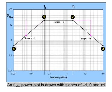
To construct a *Maximum Power* diagram, draw a horizontal line at  $S_{Max}$  amplitude between the  $f_L$  and  $f_U$  endpoints. Construct temporary points one decade below and one decade to the side of **Points 1** and **2**. Draw lines through these temporary points from **Point 1** and **Point 2** to the upper (**Point 3**) and lower (**Point 4**) frequency extremes of the plot as shown above.
