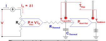
Thermal model of a capacitor in its environment.
