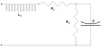
Equivalent circuit model for a ceramic capacitor.
