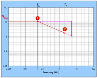
Adding a segment with a slope equal to -1/2 to the plot.
