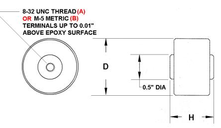
and an absence of detectable piezoelectric or electrorestrictive effects. Epoxy encapsulation provides excellent insulation resistance and a physically robust package.
