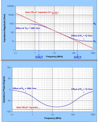
Effect of (exaggerated) R<sub>p</sub> and R<sub>s</sub> on impedance.
