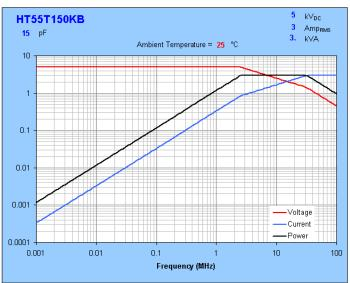
SPHT Series Ceramic Capacitors are Class 1 parts featuring high Voltage, Current and Power ratings and low self-inductance. A broad variety of these 'Power-Disk' capacitors are offered including the innovative and cost effective 'Ferris-Wheel' configuration. All SPHT capacitors have low dissipation factors. Their structure is both simple and robust, assuring a long trouble free life. SPHT Series feature a phenolic resin coating and a long flashover path.
