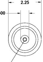
INTERNAL THREAD BOTH ENDS 10-32 UNF-2B, 1/4 DEEP (A) OR M5, 6mm DEEP (A-M)
