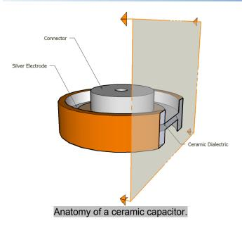
A ceramic capacitor is produced by forming and firing a ceramic cup (or back-to-back "double cup") of an insulating *dielectric* material and depositing a silver (or other noble metal) *electrode* on both sides of the 'web' or cup bottom. Copper or brass *terminals* are then soldered to each electrode and the entire structure is often encapsulated or otherwise insulated.
