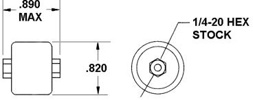
INTERNAL THREAD BOTH ENDS 6-32 UNC-2B, 5/32 MIN DEEP (A) OR M4, 4 mm MIN DEEP (A-M) OR M4, 4 mm MIN DEEP (A-SM)
